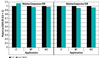
Low Temperature (LT) ): -25°F (-32°C) Evaporator, Seasonal Average Condenser (70% at 80 °F/ 30% at 105 °F), 10 °F subcool liquid, 65 °F return gas
